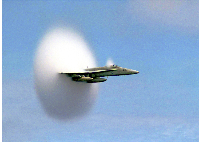
Figure 4.1: The shock wave of a supersonic airplane made visible by condensation
